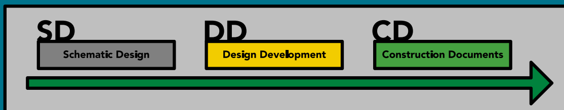
Figure 14. An Architect's Design Phases
